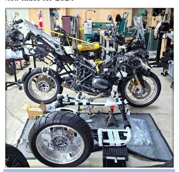
Annie Huddy has been in the process of upgrading her sidecar rides for several years. The latest, above, is having LBS adding a sidecar to her 2017 BMW R1200GS, in addition, having the shock absorbers replaced and a trail reduction modification installed. It is definitely an international rig - sidecar frame from the Netherlands, the shock absorbers from Europe, and the bike from Germany. The paint job will be local.
