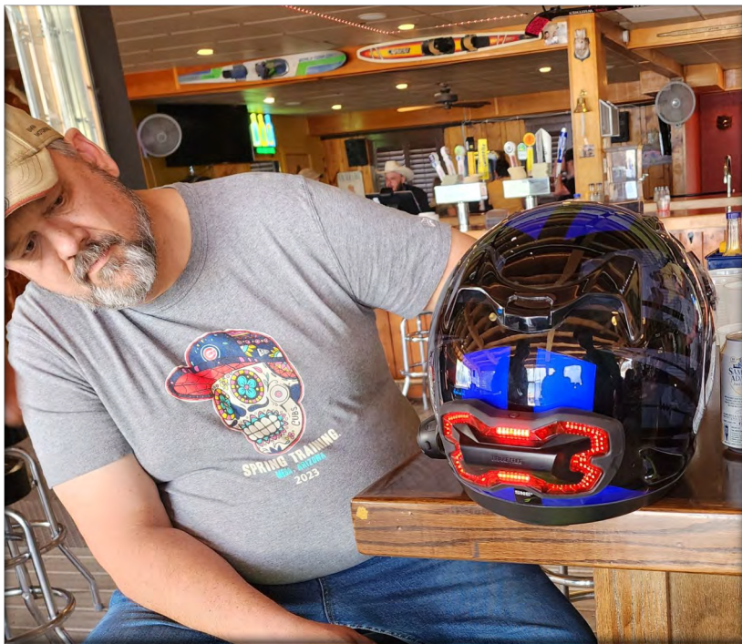
Nate Johnson inspecting Paul Smietanka's BRAKE FREE safety light. It is a wireless brake technology using a combination of gyro meter and accelerometers to detect normal deceleration, normal braking and emergency braking. It mounts on the rear of a helmet, is interchangeable and battery powered.
