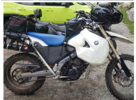
Sean rode this unusual 2007 BMW G650 X-Challenge with an aftermarket fuel tank in place of the fairing, supplementing the normal fuel tank under the seat.
