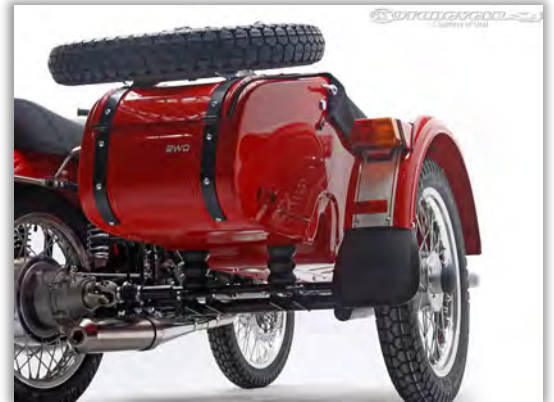
Underside of the two wheel drive configuration
