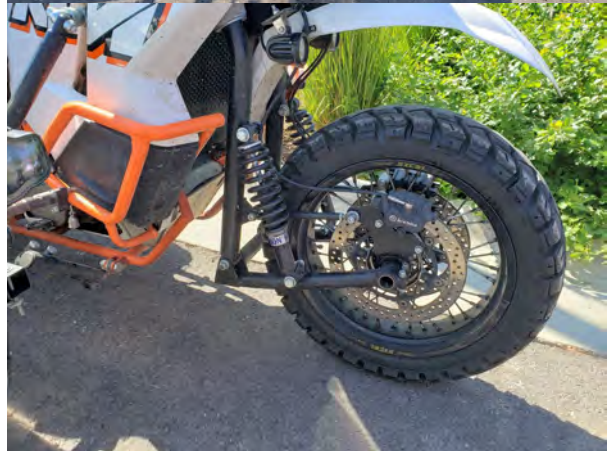
Bill's side car was specifically designed and constructed to mount on his KTM 990. Structural attachments were welded to the KTM frame for mounting points. The front suspension is also unique. I neglected to ask why this configuration was selected.
