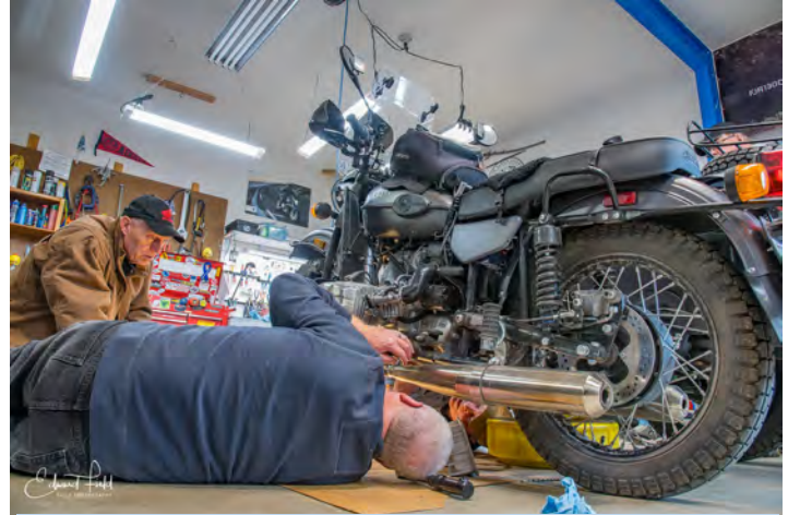
Kevin Huddy installing a new oil pan to increase the sump capacity of his 2018 Ural Gear Up. Randy Glettler, Lethbridge, Alberta looking on.
