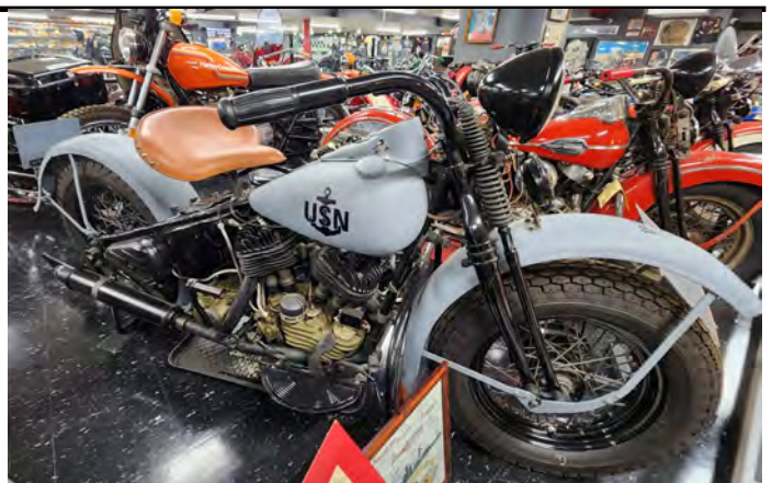
A rare 1945 - 74 cubic inch side valve Harley-Davidson with a four speed transmission, with reverse, set up for a side car. It was recovered from the Subic Bay Naval Base. Rocky Mountain Motorcycle Museum.
