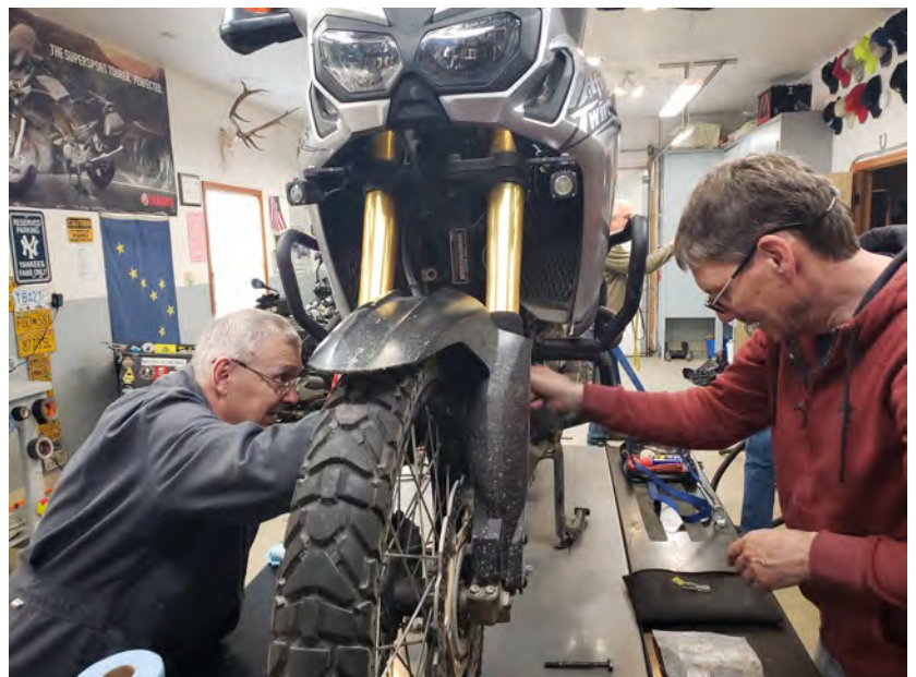
Under Ron Kitchen's skillful eye, John DiBari added a FARKLE to his Honda Africa twin, to preclude breaking off his right-side foot peg. Although a simple part, it necessitated removing the exhaust pipe to install, as seen here.
