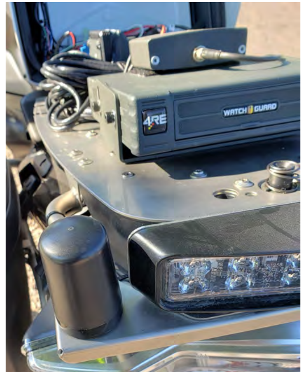
The black cylindrical piece contains the antenna that uploads data from the hard drive.
