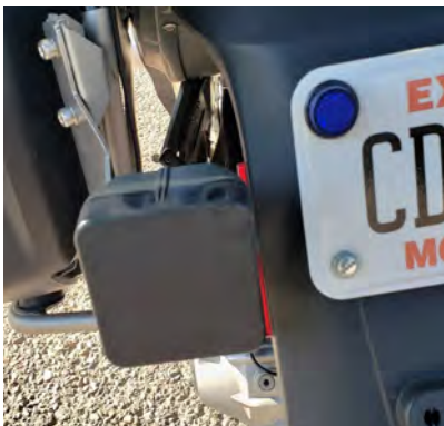
The rear facing radar. The radar system has the ability to determine the speed of an approaching vehicle, as well as a vehicle moving away from the motorcycle traveling in the same direction or in the opposite direction, both independent of the patrol motorcycle's speed.
