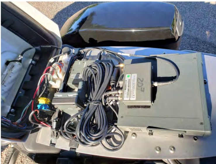
The hard drive along with the controllers for the electronics that are not related to the basic motorcycle functions.
